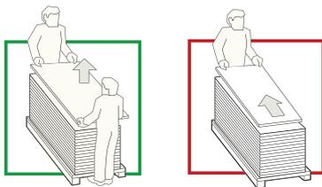
Luminare sheet must be stored horizontally, protected from moisture (without direct contact with the floor, external wall or any other damp surface). Over the sheets, an excess weight in the same dimensions as the product must be applied.
